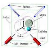
Fig. 1. Schematic View of a Horizontal-axis Washing Machine
